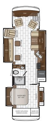
3412 34'10" Length 101.5" Width App. Overall Height 12'10" Interior Width 95.5" Interior Height 83" Grey Tank 75 gal. Sewage Tank 55 gal. Water Tank 105 gal. Propane Tank 32 gal. 35,000 btu Furnace
