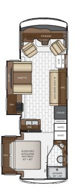
2813 Length 28'11'' Width 101.5″ App. Overall Height 12'04" Interior Width 95.5″ 80″ Interior Height Grey Tank 60 gal. Sewage Tank 40 gal. Water Tank 75 gal. Propane Tank 25 gal. 30,000 btu Furnace
