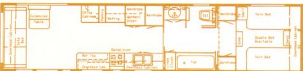
(16) 35 Walk Thru Raised Floor • Overall Length 35' 6" Approx. Hitch Weight 1500 lbs. • Approx. Dry Weight 7000 lbs.
