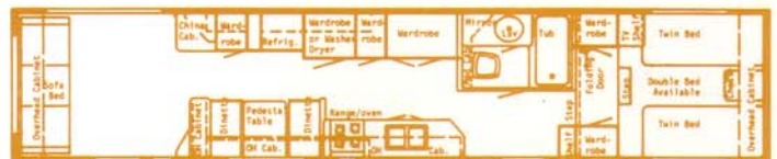
(20) 40 Front Bath Doorside Kitchen • Overall Length 39' 6" Approx. Hitch Weight 1500 lbs. • Approx. Dry Weight 7700 lbs.
