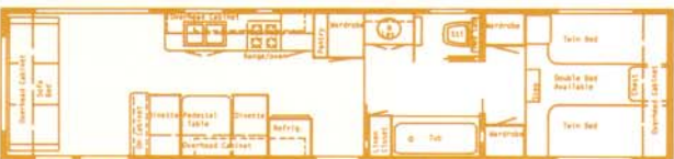
(17) 35 Walk Thru Raised Floor Dinette • Overall Length 35' 6" Approx. Hitch Weight 1500 lbs. • Approx. Dry Weight 7000 lbs.
