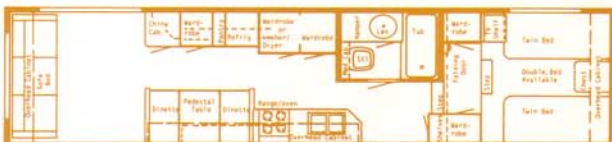
(12) 35 Front Bath Doorside Kitchen • Overall Length 35' 6" Approx. Hitch Weight 1500 lbs. • Approx. Dry Weight 6700 lbs.
