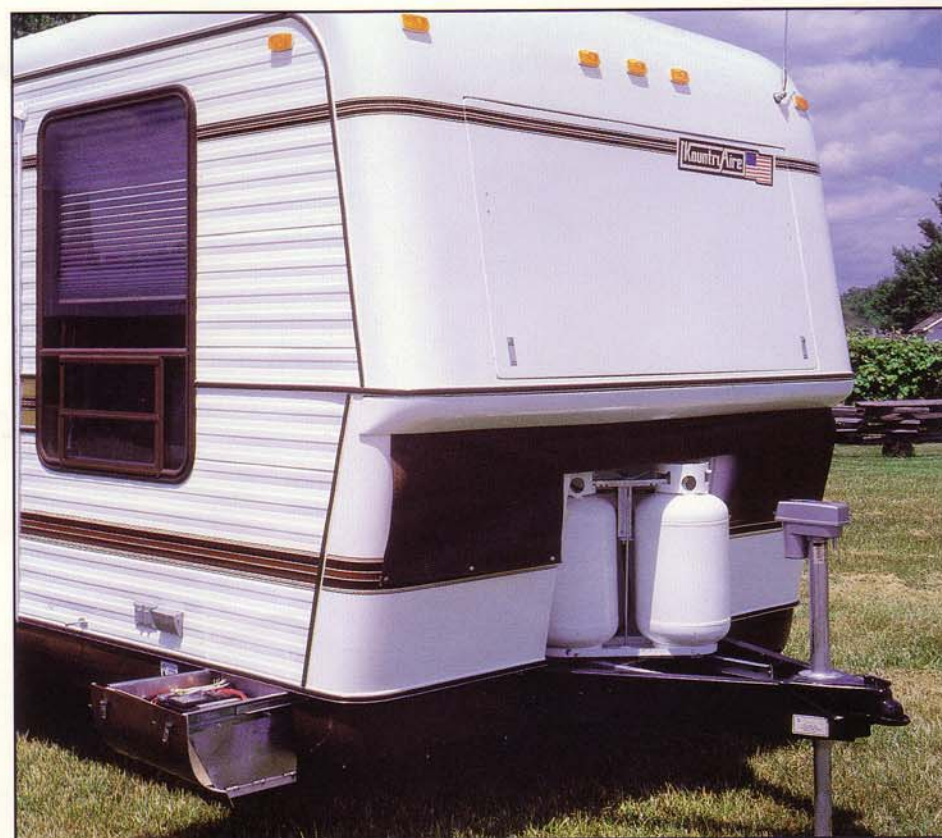
These features were originally introduced at Louisville in '85: a) a slide-out battery compartment b) a pull-down vinyl stone-guard c) an electrically-powered front awning d) a compartment to conceal the gas bottles. (Consult the spec charts to see which towable units are equipped.)
