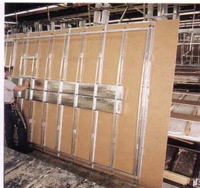
Truss style aluminum rafters are built 16" on center and central air conditioning duct work is incorporated into the design.
