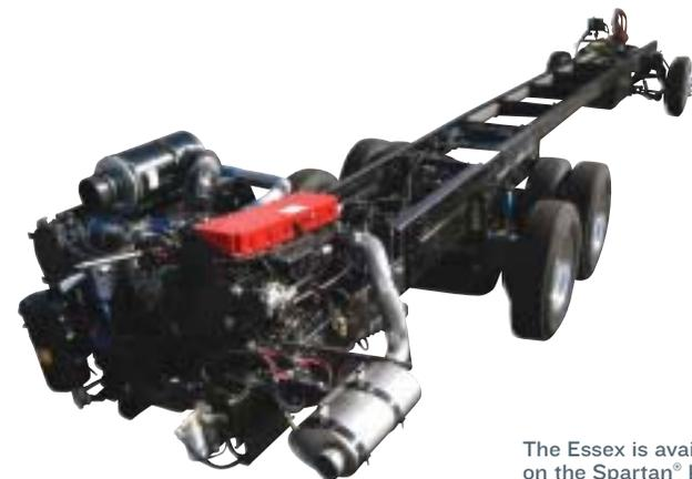
The Essex is available on the Spartan® K2 chassis with a Cummins® 500 HP ISM Engine.
