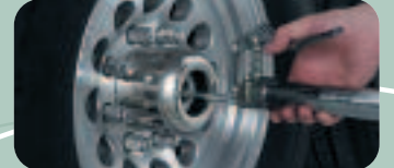
EZ Lube® axles allow RVers to periodically lubricate the bearings without removing hubs from the axles. (Shown with optional polished aluminum wheels.)
