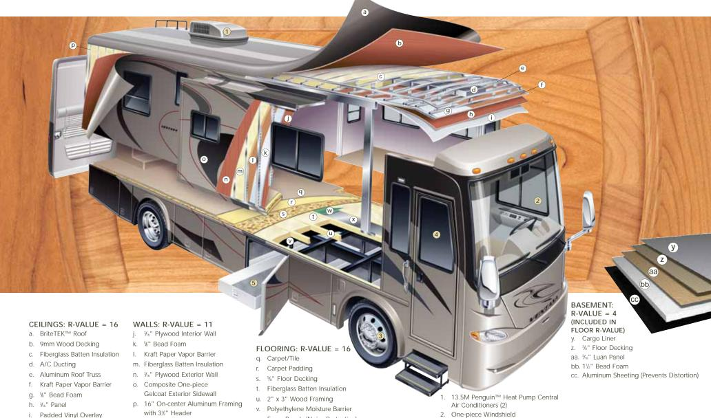
Experience RV air conditioning just like that found in site-built homes. Newmar's Total Comfort Central Air Conditioning is actually two separate, fully ducted systems: one to distribute incoming cool air, the other to quickly and effectively remove warm air from every living area.
