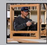
and constructed one at a time by skilled cabinetmakers. For increased stability, the frames are both glued and screwed. The finish is completed after assembly for a superior, unitized presentation.
