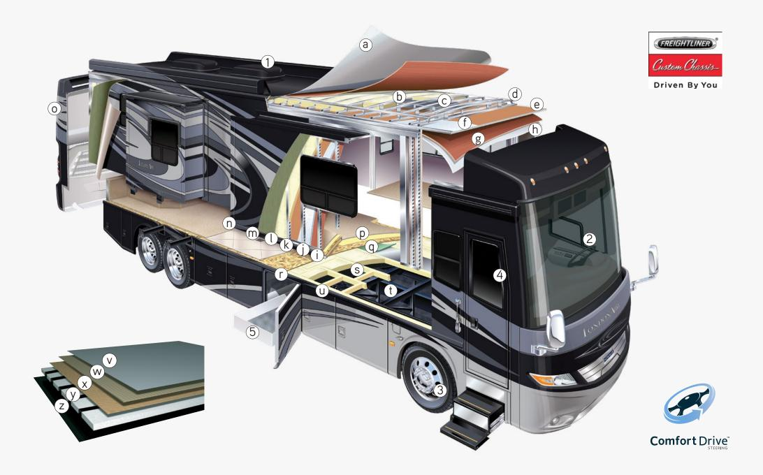
LIKE A FINE HOME, London Aire is framed 16 inches on center, allowing the best placement of outlets, switches and other components. Newmar uses only Sikaflex elastic adhesive throughout London Aire's construction – one of the strongest bonding agents available. It seals against air and
